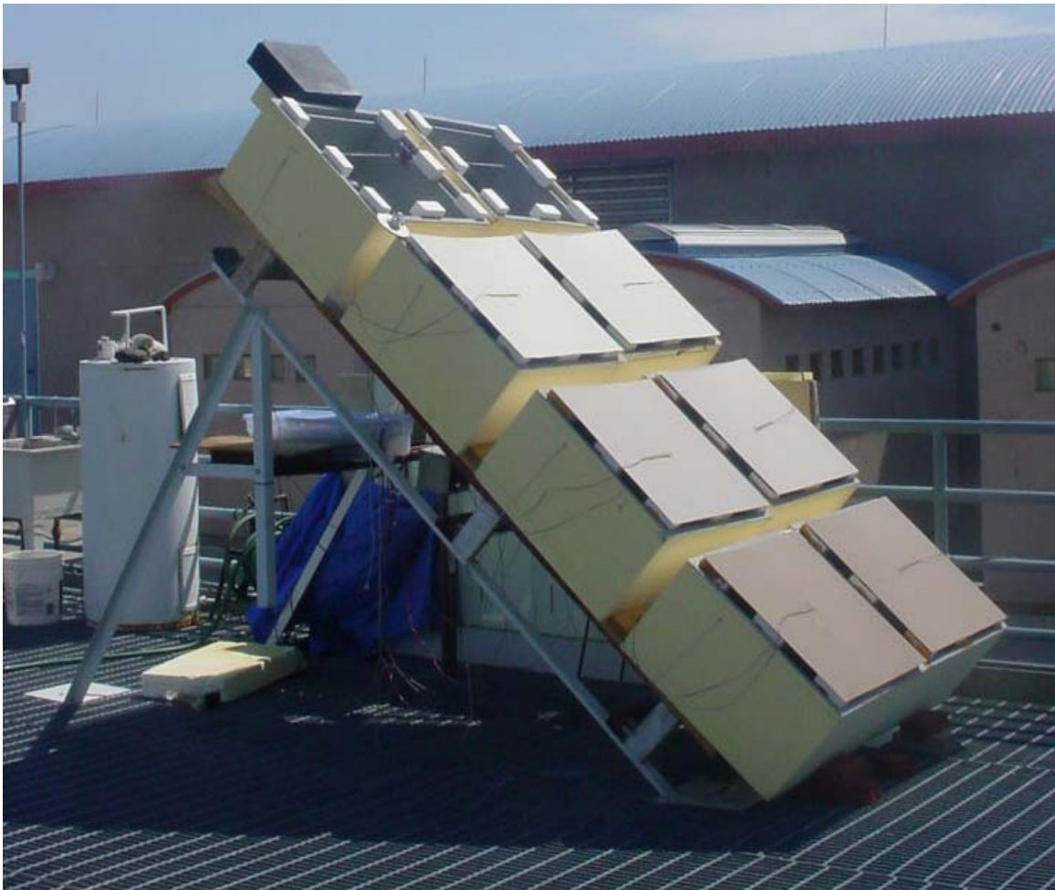
Figure 1: Test Setup for the Metal Panels and Coatings
